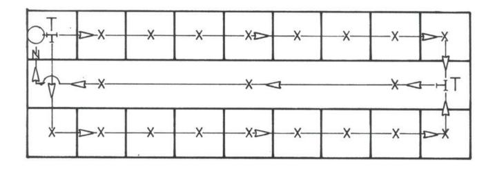
KEY: MASTER UNIT X NOZZLE ASSEMBLY N 1/4" NEEDLE (BLEEDER) VALVE T 1/4" UNION TEE DIRECTION OF FLOW
